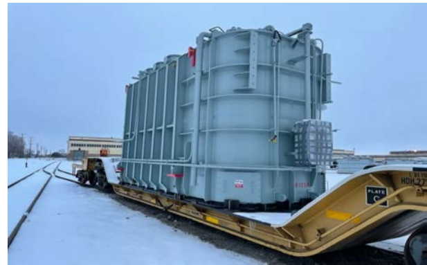
Main power transformer loaded for rail transport to Mackenzie
